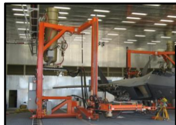
Robotics Coating Removal System
